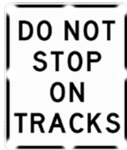
Do Not Stop On Tracks (R8-8)
