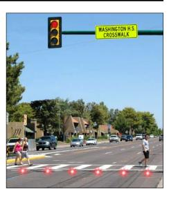
GYR inpavement lights are operated by the traffic signal light controller and display the same color: Green, Yellow or Red.
