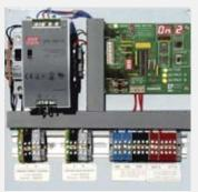
Color coded terminal blocks reduce installation time
