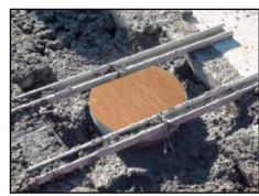
Mounting Jig Attached to Base Can
