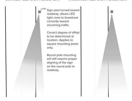
Special attention is required when mounting to existing poles. Inspection of pole placement is required to determine if LED sign will broadcast onto roadway as desired.
