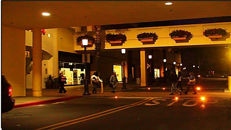
Figure 37: Warning Light System Protecting Pedestrians at Night
