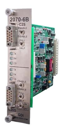
Controller and is held in place with two thumbscrews. The front panel has two M14 type connectors that are identical to the C2S and C20S connectors on the 170 Controllers. Therefore, cables made for the 300 series cabinets will work with the 2070-6B.
