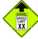
School Speed Limit Ahead Sign (S4-5)
