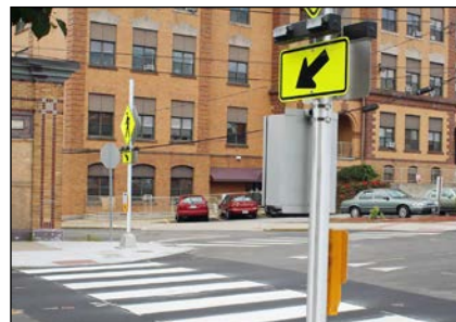
RRFBs are placed on both sides of a crosswalk in a single or double-sided (back-to-back) configuration.
