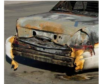
Police car destroyed from accidental combustion of pyrotechnic road flare.
