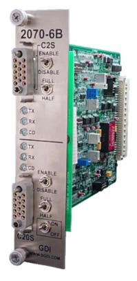
Controller and is held in place with two thumbscrews. The front panel has two M14 type connectors that are identical to the C2S and C20S connectors on the 170 Controllers. Therefore, cables made for the 300 series cabinets will work with the 2070-6B.
