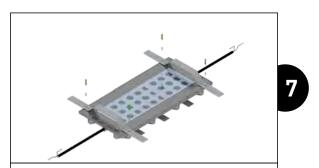
It is necessary to place the **leveling supports** on the CROSSLED product. These supports will also help in the process of handling the parts during the installation phase
