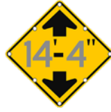
Low Clearance with Arrows Sign (W12-2)
