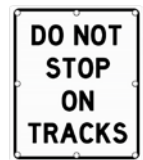
Do Not Stop on Tracks Sign (R8-8)
