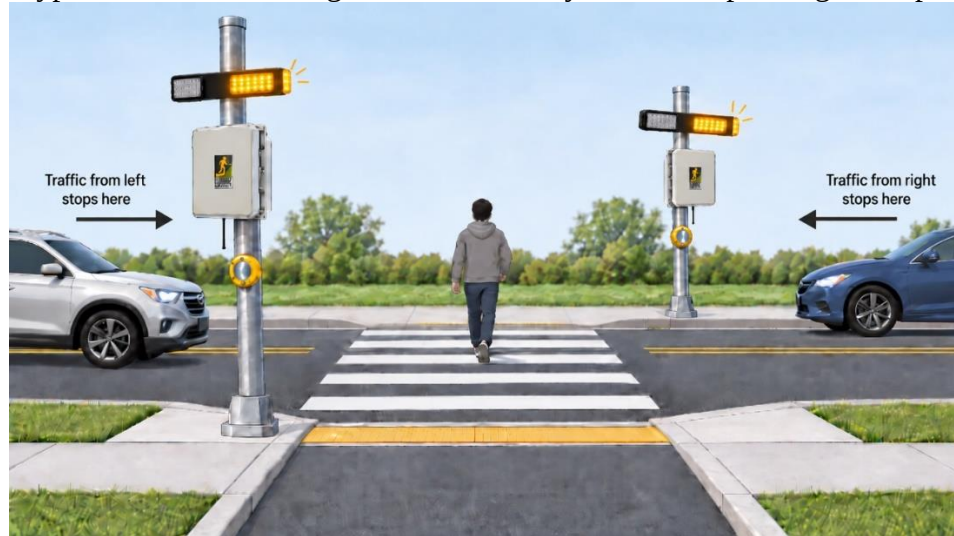
Typical TS-60S-AC Single-Sided RRFB System and Operating Principle
